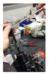
Once the old bell is dismantled, make sure that the washer of 1 mm on the nut that holds the clutch is still in place.
