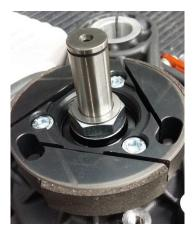
Heat the bell with a blow-dryer on both sides, about 30 secodns per side, using proper heat-resistant gloves
