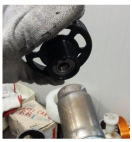
Insert it quickly on the drive shaft, pushing it until the bottom. Put the washer of 0,5 mm and reinstall the seeger.
